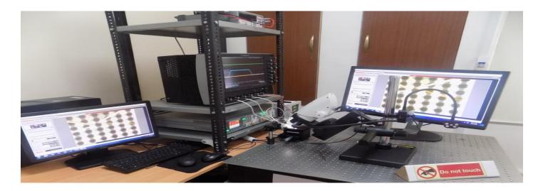
**Programmable Electrical Test (PET) System:** PET system is a custom-built, advanced programmable electrical tester, which is used to analyze time-resolved ultrafast electrical switching/transient measurements/programming of nanoscale memory devices in picosecond timescale. PET is capable of measuring transient characteristics of device within 200 ps. Further, this setup can measure a wide range of device currents (~0.5 μA to ~50 mA) in nanosecond timescale.
